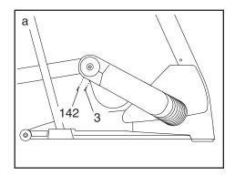
Remove the four Screws (3) from the Hood (37), and carefully remove the Hood.
